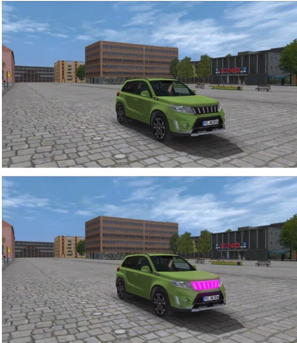
Figure 1. Screenshots of the yielding vehicle at a distance of 2.5 m from the observer without (top) and with an FBL (bottom).
